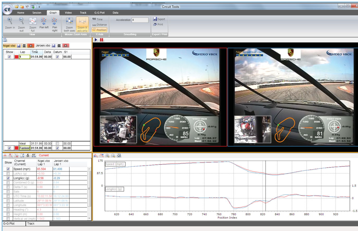
Figure 3 Entry to bus stop right-hander. Look at the g-force trace (the bottom graph). I am now braking heavily to scrub off the extra speed, whereas the other driver is coasting
