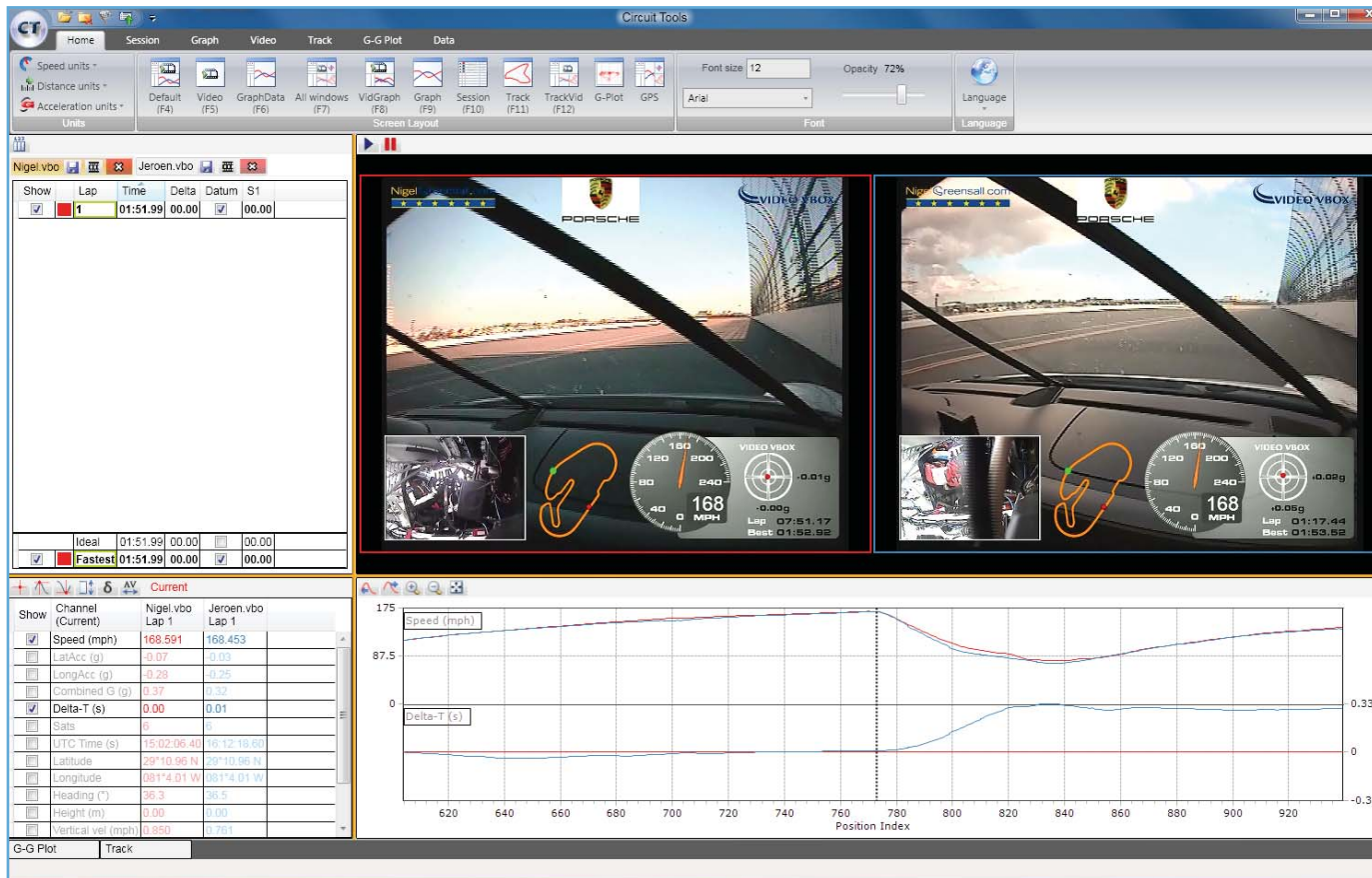
Figure 1 The Approach. As shown by the comparison video and data left (I am on the left, with the red border), both of us have the same speed at the end of the banked straight. However I am closer to the wall, which opens up my entry into the left-hander.
